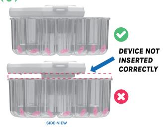
The Medesto-Go MUST sit flat securely against the Medesto-Pod when inserted correctly.
