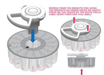
**NOTE:** If you see a gap between the Medesto-Go and the Medesto-Pod they may not be aligned properly. Lift the Medesto-Go off the Medesto-Pod and try to reinsert and realign properly.
